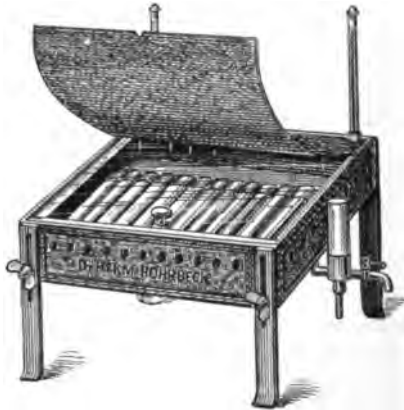
Fig. 46.—Koch's apparatus for coagulating and sterilizing blood-serum.
